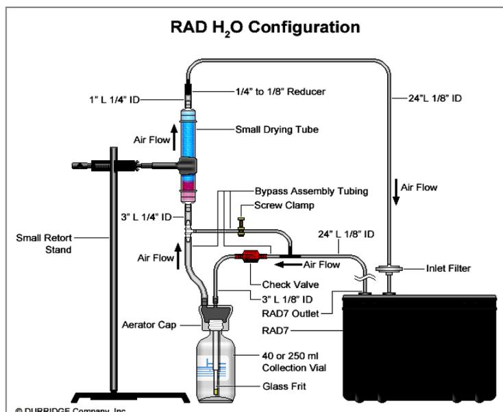
Fig.3. RAD H<sub>2</sub>O configuration diagram
